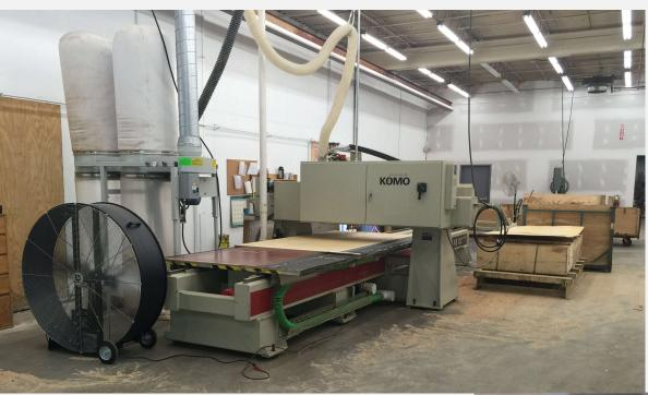
Frame components machined into "puzzle cut" components using a heavy-duty computer-controlled router to +/- 1/32" tolerance.
