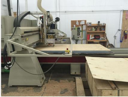
Frame components machined into "puzzle cut" components using a heavy-duty computer-controlled router to +/- 1/32" tolerance.
