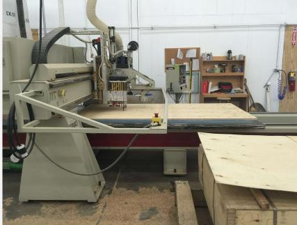
Frame components machined into "puzzle cut" components using a heavy-duty computer-controlled router to +/- 1/32" tolerance.
