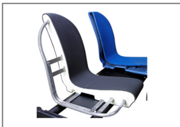
Rotationally molded vinyl seat with pressure molded foam core and steel tubular frame.
