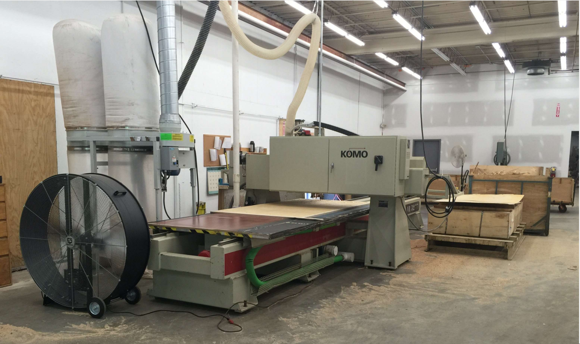
Frame components machined into "puzzle cut" pieces using a heavy-duty computer-controlled router to +/- 1/32" tolerance.
